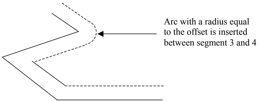
Example of Open Contour Look ahead - The following two pictures illustrate why 3 is subtracted from the segment count when determining the look ahead for open contours. In the first picture a look ahead of 4 was used so that no intersection was detected between segment 1 and segment 6. In the example, there are 7 segments. By using a look ahead of 4, problems with the blend in/out arcs will be prevented.
