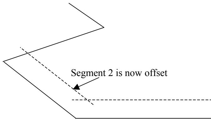
Step 3. A check for intersections is made. An intersection was found between segment 1 and 2 and the appropriate action is taken.
