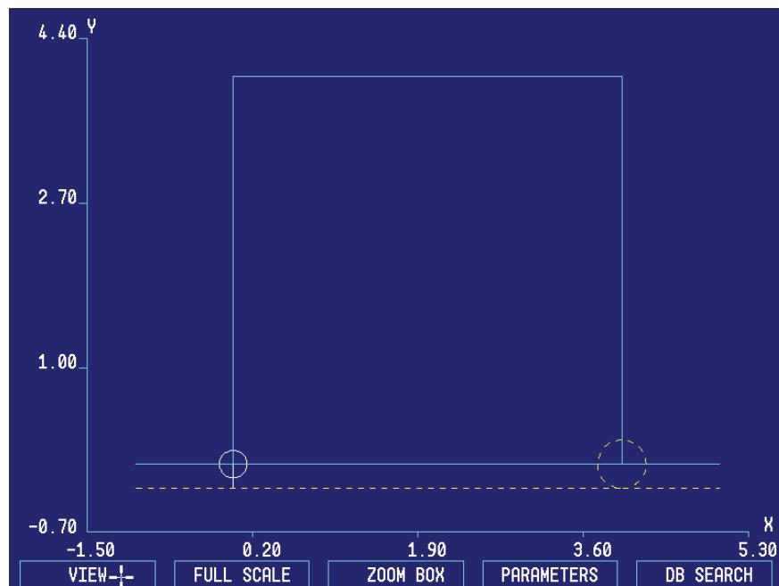
**When to use a user defined cutter comp look ahead** - The user defined cutter comp can be used with specific application problems such as contours with only a few segments that overlap or with unusual types of lead ins/out.
