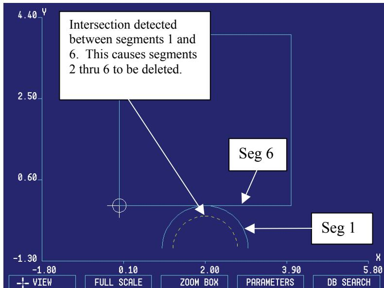
Look ahead of 5 used. When an intersection is detected, the segments between the segments that had the intersection are deleted.
