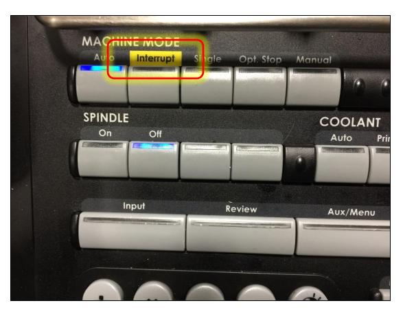
During AUTO operation, press the INTERRUPT key to cause the machine to enter the cycle interrupt mode
